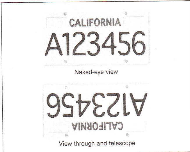
Figure 11. The view through a reflector telescope is upside down.
